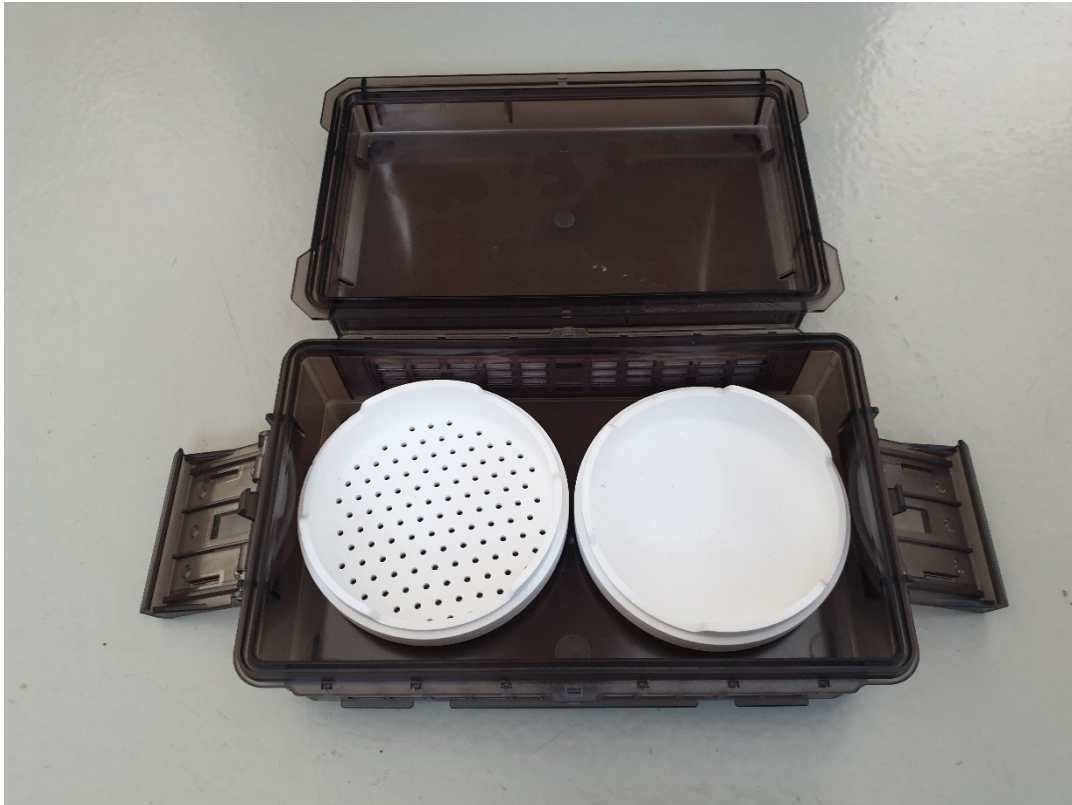
Fig. 2.3-05 2 round ceramic containers (basic cassettes) can be placed next to each other in a sterilization box
