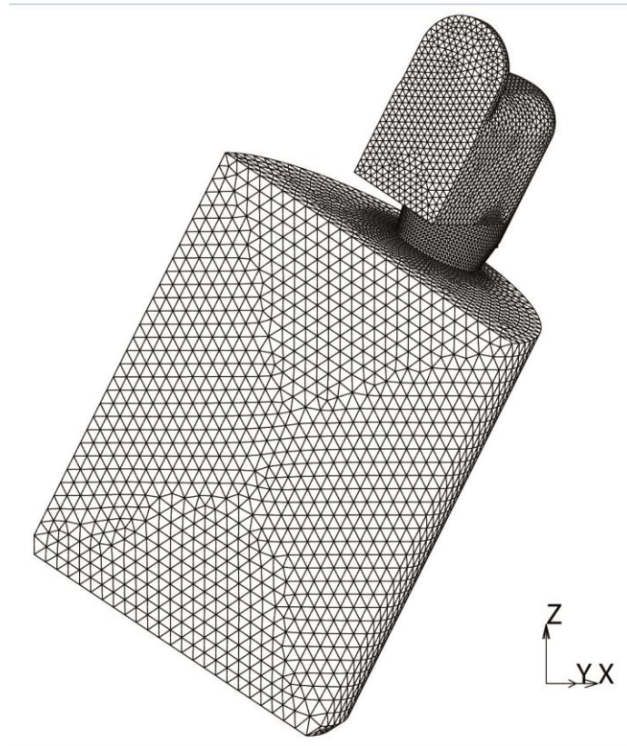
Fig. 27: FE mesh of CAD model_6 (IM-2x_R11_indi-Abut_Bridge_11G) with 1145033 elements, 1716764 nodes (half model).
